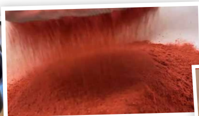
1 Freeze-dried fruits are processed into powder and finely sieved.
